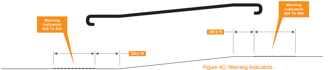
Figure 4C: Warning Indicators - Ramps. Side elevation where top and bottom of ramp leads to an open area
